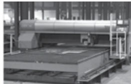
LASER BURNING PRECISION CUT UP TO 1" THICK PLATE \pm 0.10
